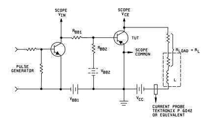
$\begin{array}{l} R_{BB1} \,=\, 10\Omega \\ R_{BB2} \,=\, 100\Omega \\ L \,=\, 0.3 \ mH \\ R_L \,=\, 0.1\Omega \\ V_{CC} \,=\, 10 \ V \ dC \\ I_C \,=\, 10 \ A \\ V_{BB1} \,=\, 10 \ V \ dC \\ V_{BB2} \,=\, 4 \ V \ dc \end{array}$
